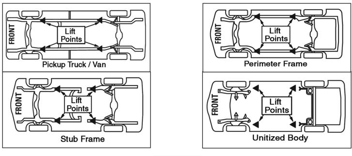
Make sure vehicle is neither front nor rear heavy. Center of balance should be midway between adapters as shown below.
