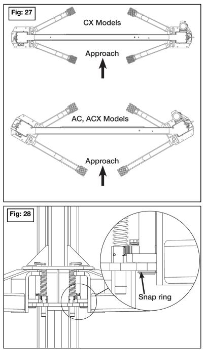
7. Ensure that the arms do not move when a force of approximately 100 pounds or less is applied laterally to the fully extended arms. 8. Adjust the gear ring on the arm as necessary to ensure smooth operation and solid engagement of all four arm restraint pin assemblies with the arm restraint gear ring.
