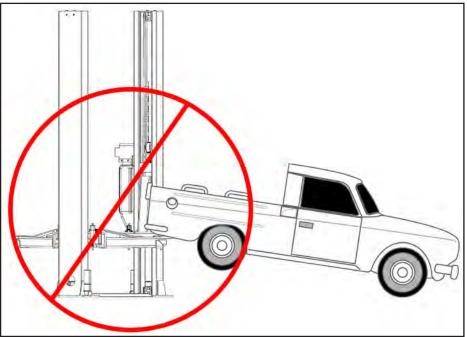
NEVER LIFT ANY VEHICLE IN ANY MANNER WITH LESS THE ALL FOUR (4) ARMS. RATED CAPACITY OF EACH LIFT ARM IS NO GREATER THAT ONE FOURTH (1/4) OF THE OVERALL LIFT CAPACITY.
