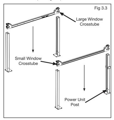
4. With the posts standing and the cross tubes in position, install the Safety Ladders. Pass the ladders through the post openings and drop down through the Slide Block guide slots on the crosstubes until the ladders come to rest on the base plates. If bolting, DO NOT BOLT posts down at this time. (See Fig. 3.4)
