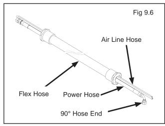
6. Install the end of Flex Hose with the Straight Fitting on the Hydraulic Hose into the hole in the Powerside Runway adjacent to the Power Unit. Install the end of the Flex Hose with the 90° Fitting on the Hydraulic Hose in the Flex Hose Bracket Assy. Tighten the plastic nuts securely. (See Fig 9.7)
