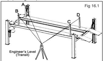
5. Beginning with the "A" position, sight the Level to the target and mark the number or the graduation on the inch scale of the target that aligns to the crosshairs of the Level. (See Fig. 16.1)
