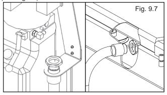
7. Connect the hydraulic hose and air line as shown below making sure the hydraulic hose passes through the retaining rings. MAKE SURE HOSES ARE KEPT CLEAR OF CABLES. There will be one air line hose left unconnected in this step. This air line will be used to activate the pneumatic safety locks in the next step. See page 19 for Compression Fitting instructions. (See Fig. 9.8)
