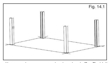
with proper clearances around and overhead. (See Fig 14.1) 2. Using the base of the frame as a guide, drill each anchor hole in the concrete approximately 4" deep using a rotary hammer drill and 3/4" concrete drill-bit.
