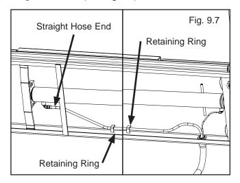
8. Connect the straight end of the Power Unit Hydraulic Line to the 90° Power Unit Fitting. Connect the Return Air Line to the 90° Air Fitting. There will be one air line hose left unconnected at this time. This air line hose will be used to activate the pneumatic safety locks on the next page. (See Fig. 9.9)
