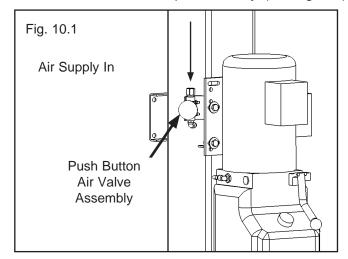
2. Route the air line that was left unconnected in Step 9 to the 90° Air Line Compression Fitting of the Push Button Air Valve Assembly. (See Fig 10.2)
