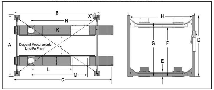
**NOTE:**TO CHECK IF LIFT IS SQUARE, DIAGONAL MEASUREMENTS OF POSTS AS SHOWN ABOVE MUST BE EQUAL
