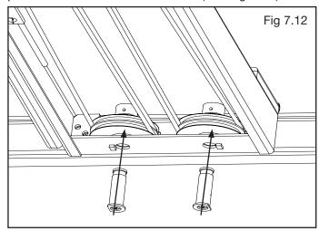
5. Install the Socket Head Cap Screws though the Sheave Axle Collars. (See Fig. 7.13)
