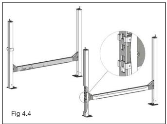
3. The posts and crosstubes will now be in position and spaced properly for the ramps. Be very careful not to disturb the posts and crosstubes at this time as they may tip over causing personal injury or harm.
