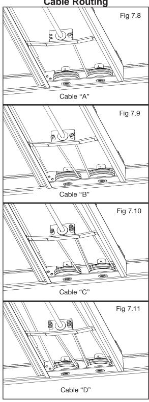
4. With the cables properly routed, hold the sheaves in position and install the sheave axle. (See Fig. 7.12)
