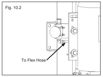
3. Once the air line has been connected with the Push Button Air Valve, cut the air lines to length by following the Safety Air Line Routing diagram located on Page 20 and connect female branch "tee" fittings where needed.
