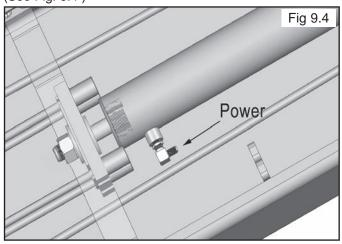
4. Install the 90-degree Air Line Compression Fitting in the port at the base, pinned end of the Cylinder. On the pipe thread side of the Fitting, it is recommended to use Teflon Tape or pipe sealer. (See Fig. 9.5)
