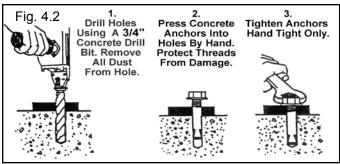
Secure Power Unit Stand to the floor using two 3/4" anchor bolts supplied.
