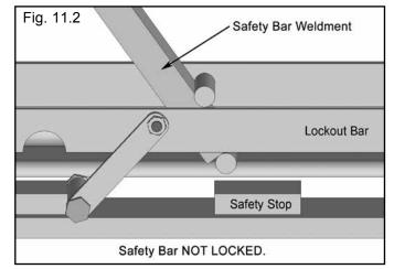
5. Push LOWERING valve handle to lower. Note: Both SAFETY LOCK release and LOWERING valve handles must be held down simultaneously to lower lift. Do not override self-closing lift controls.
