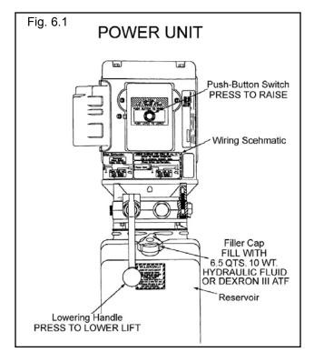
3. The standard power unit for your lift is 110 volt, 60HZ, single phase. All wiring must be performed by a certified electrician only. SEE WIRING INSTRUCTIONS AFFIXED TO MOTOR FOR PROPER WIRING INSTRUCTIONS.
