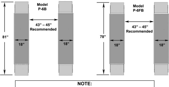
The maximum recommended width between pads is 45". Consult the factory for applications that require installations wider than 45".
