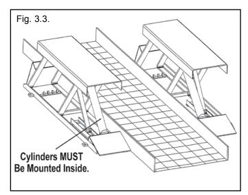
5. It may be necessary to remove the tire rail adjacent to the lift pad and overhang the edge of the rail to maintain the recommended width between pads.
