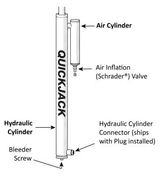
The components of the Air and Hydraulic Cylinders are:
