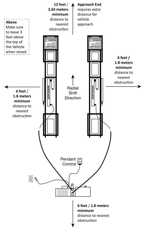
Vehicle approach must be opposite Power Unit. Do not drive Vehicle on Hydraulic Hoses, Power Unit, or QuickJack Frames. **Always** place the Power Unit and Pendant in a position so that the Operator has a clear view of **both Frames** while operating the QuickJack.
