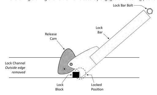
Not to scale. Not all components shown. Shows Release Cam and Lock Bar in Locked Position.
