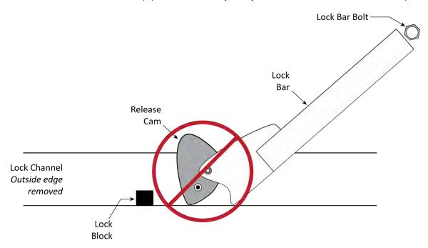
Not necessarily to scale. Not all components shown. Release Cam shown in the Up position, which must be changed to the Down position before lowering.
