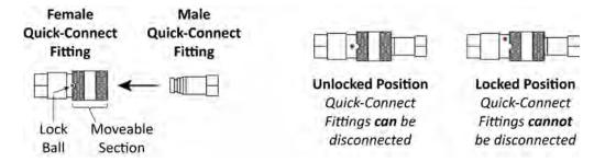
**To lock a connection**: Push the Male Quick-Connect Fitting into the Female Quick-Connect Fitting, then turn the Moveable Section so that the Lock Ball is not opposite the Notch.
