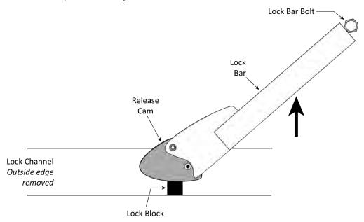
Not drawn to scale. Not all components shown. Release Cam shown on top of the Lock Block.
