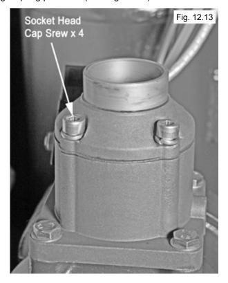
3. Remove and replace the Valve Body Top Gasket. Remove the Valve. (See Fig. 12.14)
