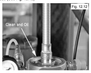
6. Screw the new Air Oil Filter on clockwise and hand tighten only.
