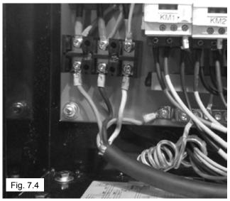
3. Connect the Power Source Wires to the incoming Power Terminal Block. (See Fig. 7.4)
