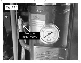
2. Confirm the pressure has been bled off by reading Pressure on oil Separation Tank. (See Fig.12.2)
