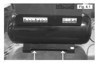
**Never** use the wood shipping pallet for mounting the compressor.
