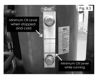
3. Fill with PowerCool Synthetic Air Compressor Lubricant if necessary and inspect the O-Ring on the Oil Fill Plug before tightening.
