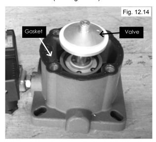
4. Inspect the white seal on the Valve for damage or cracks. Replace if damaged. (See Fig. 12.15)
