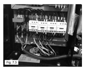
2. Route the power cable through the bottom of the Power Control Box and to the Terminal Block as shown below. (See Fig. 7.3)
