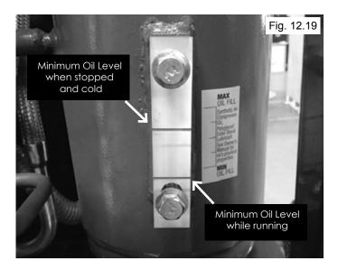
8. Start the compressor. Check the oil level while running and add oil as required. Check again after compressor has be running for about 30 minutes and stopped for 30 minutes. If oil level is low, add Oil as needed.
