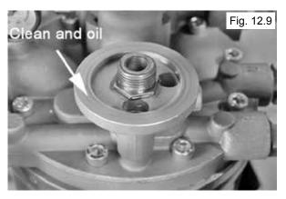
4. Screw the new Oil Filter on clockwise and hand tighten only.
