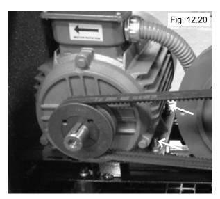
3. Using a straight edge or square and or level, adjust the motor until the Motor pulley and Air End Pulley are in the same vertical and horizontal plane. Shims may be required. (See Fig. 12.21)
