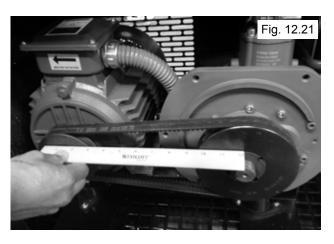
4. Tighten the Mount Bolts and adjust Pulley Tension as described in procedure below.
