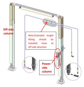
7.To install the safety cable, refer to manual guidance
