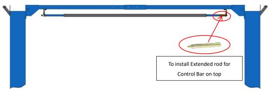
5.To install longer version cable 9.52\*10198mm:Both two sides carriage should be sync lifted and keep the same height, before install the cables, refer to manual guidance)
