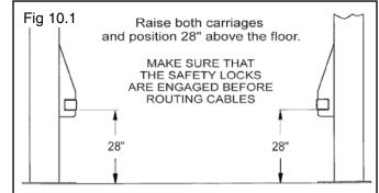
2. With the carriages locked at 28" off the floor, route the threaded end of the equalizer cable across to the opposite side base plate sheave and up through the carriage. (See Fig. 10.2)
