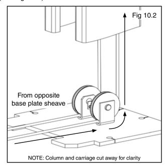
3. Route the threaded end up and over the Top Plate sheave and back down to the carriage and reinstall sheave. (See Fig. 10.3)
