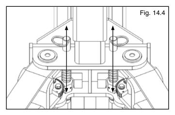
6. Ensure that the arms do not move when a force of approximately 100 pounds or less is applied laterally to the fully extended arms.
