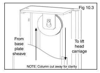
4. Insert the threaded end of the cable through the hole on top of the carriage. Place M18 washer and M18 Nylock nut on threaded cable end. Tighten cable nuts until taut, checking that both cables have equal tension. (See Fig 10.4)
