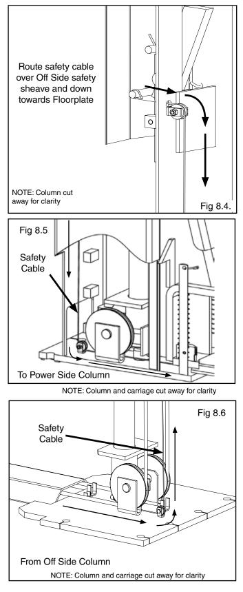
5. Route the cable the same way as on the Power Side going up the Column and over the safety cable sheave.
