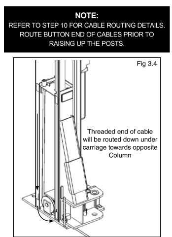
NOTE: Portions of Carriage and Column cut away for clarity
