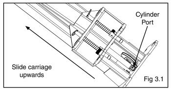
2. Install a 1/4" NPT straight fitting into each cylinder port using teflon tape then temporarily remove the cable sheaves located at the inside bottom of each Column by first removing the hex head bolts, and then by removing the sheave pin. (See Fig 3.2)
