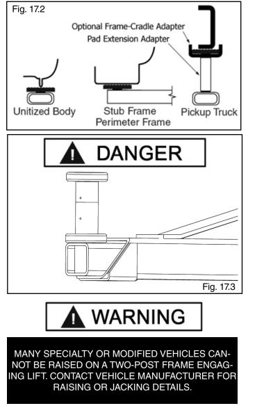
4. Position vehicle for proper weight distribution arms under vehicle to allow adapters to contact at the manufacturer's recommended pick up points.
