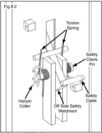
2. From the Off Side Column insert the non-looped end of the safety cable through the hole located to the right of the Off Side safety weldment. (See Fig 8.3)
