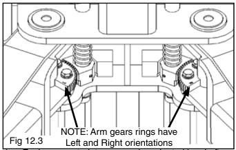
4. Each arm restraint gear can be oriented in a Left or Right configuration on the arms. Each arm and arm restraint gear must be positioned in the proper location in the lift head. (See Fig. 12.4 & 12.5)
