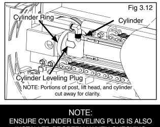
ENSURE CYLINDER LEVELING PLUG IS ALSO INSTALLED PROPERLY WHEN CHECKING ALIGNMENT OF CYLINDER AND CYLINDER RING 9. Uncoil cable and route cable around the Top Plate sheave and coil the remaining cable up and leave it in the post above the lift head. (See Fig 3.13)
