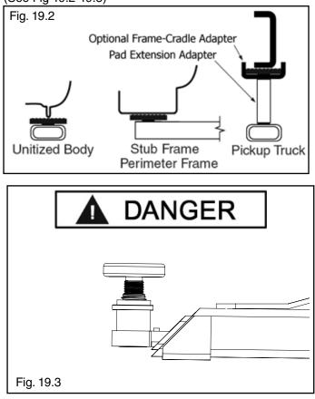
3. Some vehicles may have the manufacturer's Service Garage Lift Point locations identified by triangle shape marks on the underlift head (reference ANSI/SAE J2184-1992). Also, there may be a label located on the right front door jamb area showing specific vehicle lift points.
