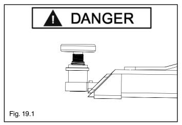
• **DO NOT** block open or override self-closing lift controls; they are designed to return to the "Off" or Neutral position when released.
