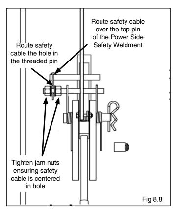
8. Operate the Power Side safety handle, check for proper operation of both safety assemblies and adjust cable tension as required.
