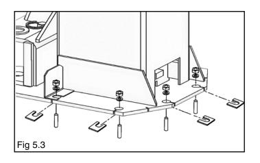
6. With the foot guards, shims and anchor bolts in place, tighten by securing the nut to the base then turning 3-5 full turns clockwise (90 ft-lbs.). **DO NOT** use an impact wrench for this procedure. (See Fig. 5.4)
