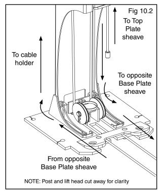
3. Route the threaded cable end to the opposite post's base plate sheave. Wrap the cable around the opposite post's Base Plate sheave and reinstall sheave. (See Fig. 10.2)
