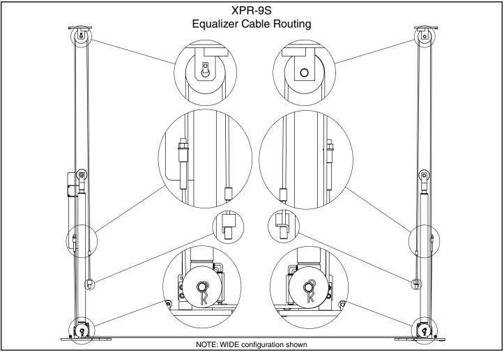
2. With the lift heads locked at 28" off the floor, uncoil the equalizer cables and route the threaded end of the equalizer cables towards the Base Plate sheave. Wrap the cable around the base plate sheave and reinstall sheave. (See Fig. 10.2)
