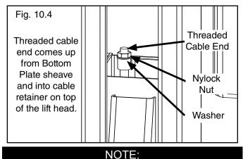
THERE WILL BE INITIAL STRETCHING OF THE CABLES AND/OR WITH INCREASED LOADS. ADJUST THE CABLES AS OUTLINED ABOVE A WEEK AFTER FIRST USE, THEN EVERY THREE TO SIX MONTHS THEREAFTER DEPENDING ON USAGE AND/OR TO COMPENSATE FOR STRETCH.
